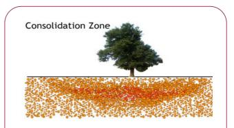
Although the soils are saturated due to winter recovery, the clay particles will have consolidated and the 'memory of desiccation' could be revealed by the penetrometer, but missed by the suction test.
